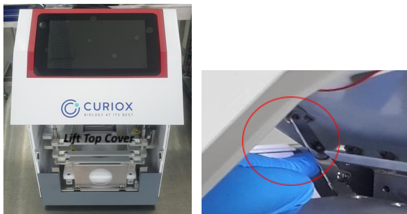
Figure 3-1: Lift the machine top cover (left) and lock in the open position (right).
